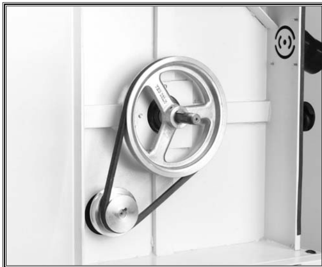
Figure 28. Speed pulley (lower wheel removed for clarity).
